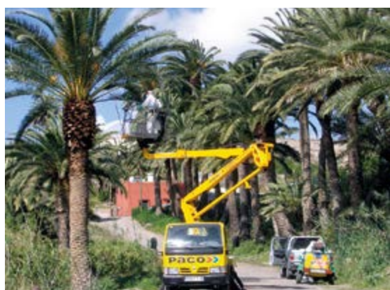
Figure 85. Truck mounted elevator with platform to treat the crown of the Canary Island palm
