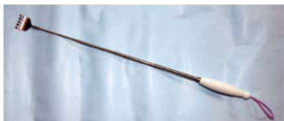
Figure 23b. Telescopic probe, partly extended
